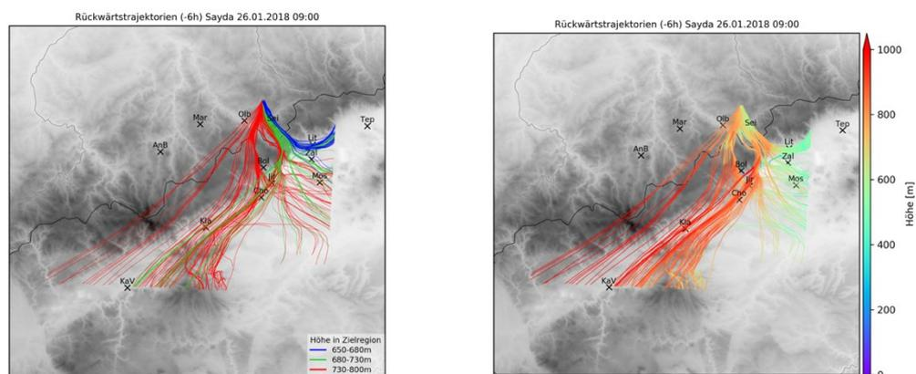
**Figure 2:** Backward trajectories (6 hours back) for Sayda, Germany, on 26/01/2018 09:00. Left: Coloured according to height at the target area (blue: low, green: medium-high, red: high). Right: Coloured by absolute altitude. (Orography data: *NASA SRTM v4.1.*)
