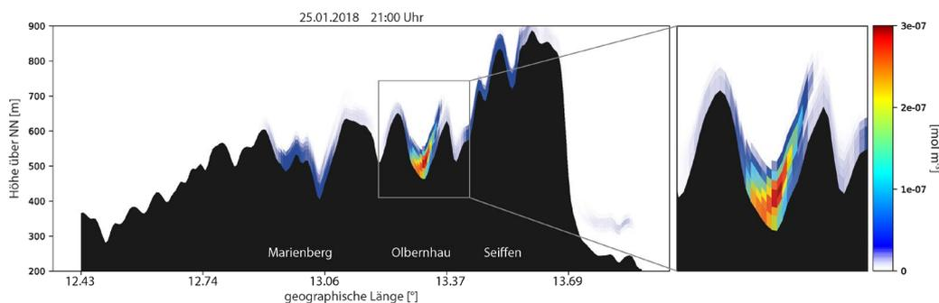
**Figure 4:** Vertical sections through the model area on a line from Marienberg via Olbernhau to Seiffen on 25/01/2018 21:00 (left, cf. Figure 5) and the section enlarged by Olbernhau (right). The height of the concentration refers to an assumed constant source strength of the point sources of  $1 \text{ mol s}^{-1}$ .
