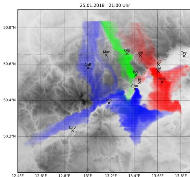
**Figure 5:** Concentration of the tracers from the sources CHO (blue), BOL (green) and ZAL (red) on 25/01/2018 21:00. Low concentrations are shown transparent, high concentrations opaque. The dashed line marks the position of the vertical profile in Figure 4.
